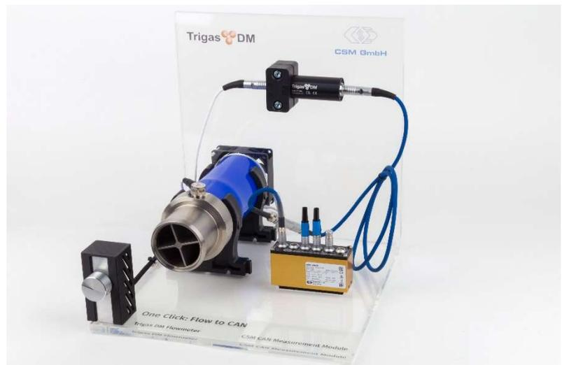
In addition to the linearized flow output signal, transmitted is also the Transducer Electronic Data Sheet (TEDS) of the sensor. The measuring point name, calibration data and flow measuring ranges are included. When the sensor is connected to CSM's new AD-Scan MiniModule (ADMM 4 CXS), all information is converted to a CAN bus signal.
