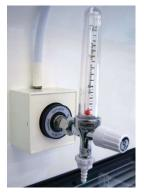
A rotameter has a floating indicator in a graduated tube.
