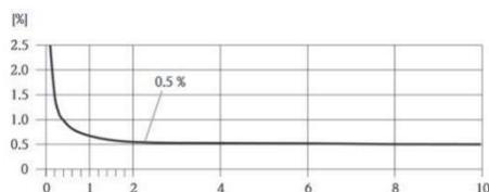
Furthermore, the Magnetic flowmeter size was such that in this application it would be used in the far low end of its specified range. Below 1 m/s, mostly due to zero-shift characteristics, the error curve of these devices diverges rapidly.
